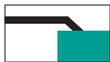
Inset: The rim of the sink after installation appears on the worktop.
